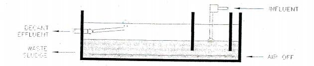
Receives Influent Continued BOD<sub>5</sub> Oxidation Sludge is Wasted Decants Effluent Denitrification
