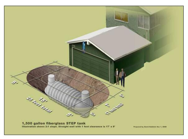
Figure 2: STEP Excavation
