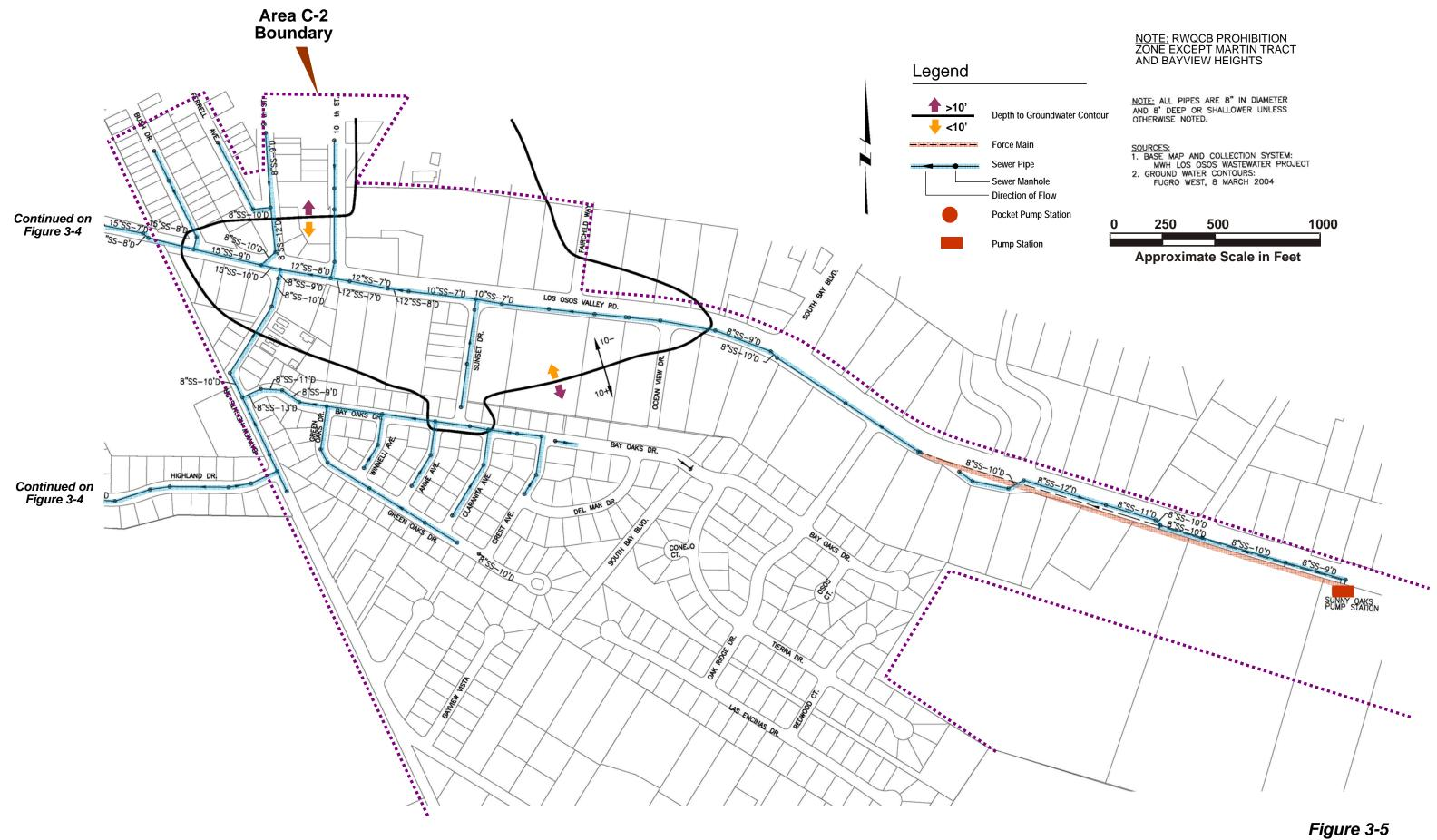
Figure 3-5 Collection System Layout – Area C-2 Los Osos Wastewater Project EIR
