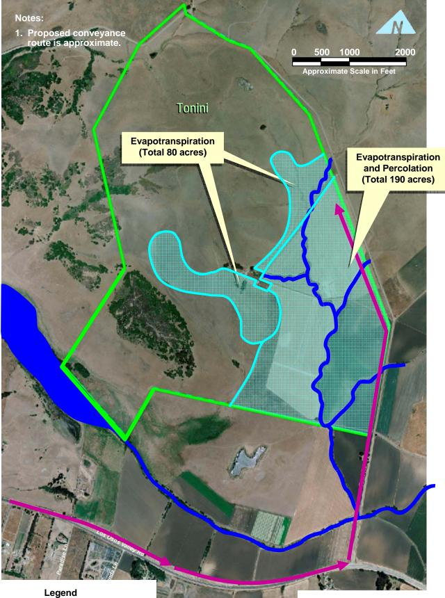
Proposed Conveyance Property Boundary Spray Field Drainage Channel
