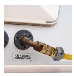
Fill line to non-portable tank with a quick disconnect coupler
